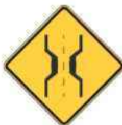
Two-lane narrow bridge or culvert ahead. Approach with caution.
