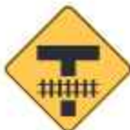
Railroad before "T" Intersection
