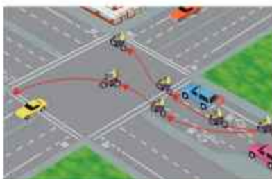
Intersections with special lanes for bicyclists.
